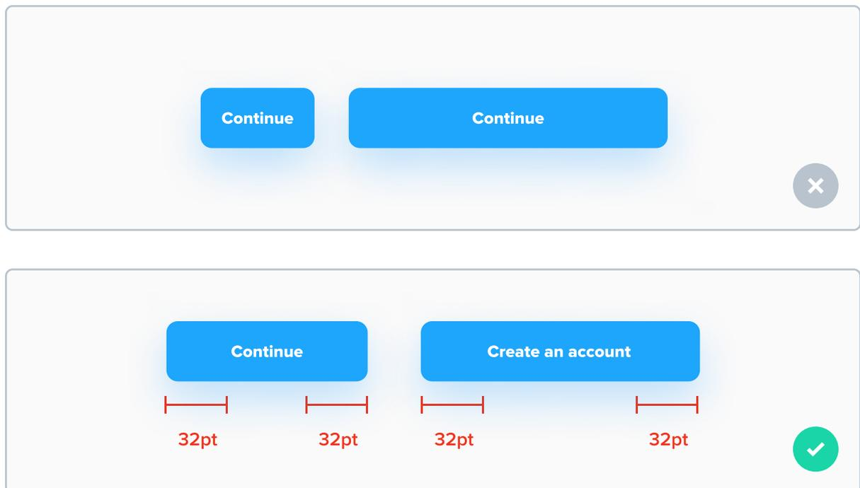
As you can see above, button width should depend on the width of the text inside of it, at least for web interfaces. For mobile interfaces, in 99% of cases buttons cover the whole width of the screen (excluding the margins).
